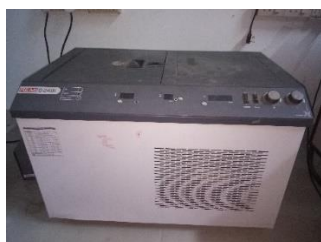
High Speed refrigerated centrifuge machine with stabilizer (REMI)
