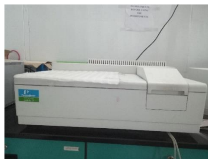
Double Beam UV-Visible Spectrophotometer with Peltier Temperature Control System from 0-100C (Perkin Elmer lambda-35)
