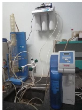
De-ionise Water Purification System (Thermofisher, 6 litres/hr)
