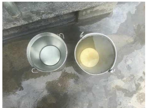
Image showing the difference between from the left to the right Treated water by the water treatment plant and untreated pond water.
